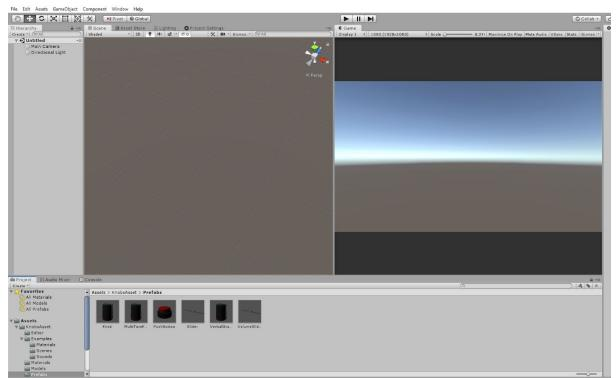
The basic versions of the prefabs with standard settings are "Knob", "PushButton" and "Slider". Drag the prefabs into your scene, then position and scale them to where you want them to be.
